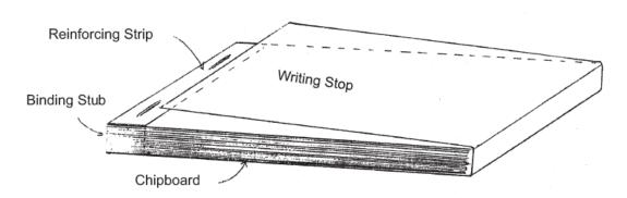
CONSTRUCTION: Bind \_\_\_\_\_\_\_part sets per book. Matchbook style cover with reinforcing strip on top. (May wrap around binding stub or not at contractor's option.) Two wire stitches through binding stub. A piece of chipboard or equal, approximately .020" thick to be placed between bottom set and cover. Cover to fold around to form writing stop. SCORE cover at all folds.
