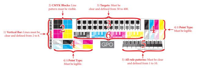
This is the GPO Resolution Target, it must be imaged at 100%, along with the Idealliance G-7 Target on all proofs. To ensure your proof is acceptable for Hi-Resolution Ink Jet, it must pass the following criteria:
